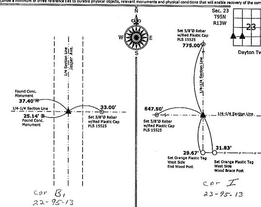
1.) SW Corner NW 1/4-SW 1/4 Section 23-95-13 Set 5/8"Ø rebar w/2"Ø aluminum cap PLS 15525
