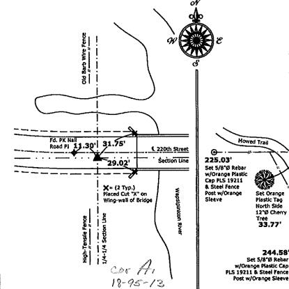
1.) Southwest Corner SE 1/4-SE 1/4 Section 18-95-13 Set Survey Mark Nail w/Stainless Steel Washer PLS 19211
