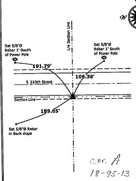
1.) South 1/4 Section 18-95-13 Set 5/8"Ø rebar w/2"Ø aluminum cap PLS 19211
