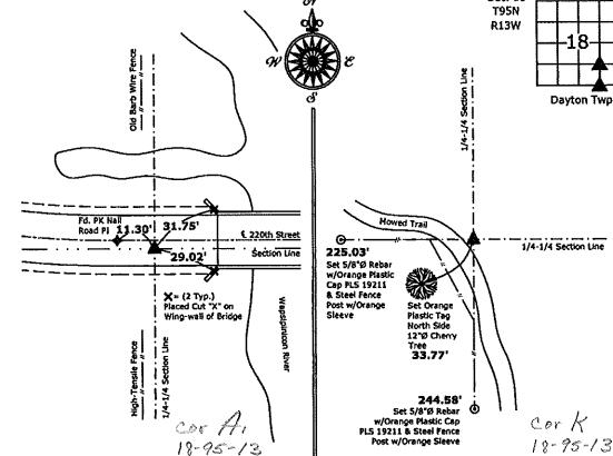
1.) Southwest Corner SE 1/4-SE 1/4 Section 18-95-13 Set Survey Mark Nail w/Stainless Steel Washer PLS 19211
