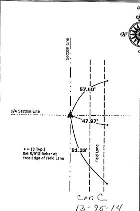
2.) Northwest Corner NE 1/4 SW 1/4 Section 18-95-13 Set 5/8\*Ø rebar w/2\*Ø aluminum cap PLS 19211
