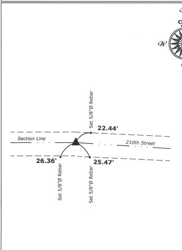
1.) S 1/4 Corner Section 8-95-13 Fd. Granite Stone w/1" Square Iron Bar on East side, 24" deep Set 5/8"Ø rebar w/2"Ø aluminum cap PLS 15525 Over Stone
