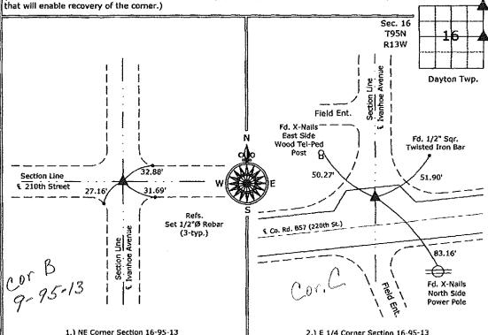
1.) NE Corner Section 16-95-13 Fd. 5/8°Ø rebar w/Yellow Plastic Cap RLS 7549 2.) E 1/4 Corner Section 16-95-13 Fd. PK Nail
