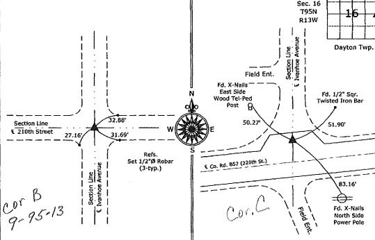
1.) NE Corner Section 16-95-13 Fd. 5/8°Ø rebar w/Yellow Plastic Cap RLS 7549 2.) E 1/4 Corner Section 16-95-13 Fd. PK Nail
