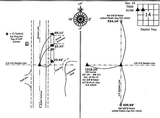
1.) Northwest Corner SW 1/4 - NW 1/4 Section 14-95-13 Set 5/8°Ø rebar w/2"Ø aluminum cap PLS 15525
