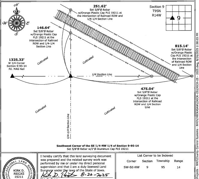
Southwest Corner of the SE 1/4-NW 1/4 of Section 9-95-14 Set 5/8"Ø Rebar w/2"Ø Aluminum Cap PLS 19211
