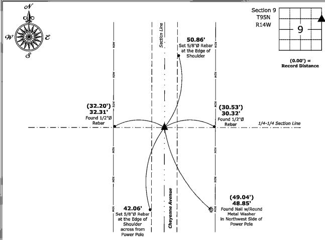
Northeast Corner of the SE 1/4 - NE 1/4 of Section 9-95-14 Found 1/2"Ø Rebar
