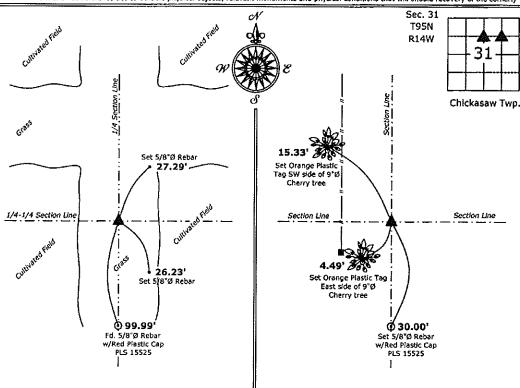
1.) Northwest Corner SW 1/4 - NE 1/4 Section 31-95-14 Set 5/8°Ø rebar w/2°Ø aluminum cap PLS 15525 2.) Northwest Corner SE 1/4 - NE 1/4 Section 31-95-14 Set 5/8\*Ø rebar w/2\*Ø aluminum cap PLS 15525
