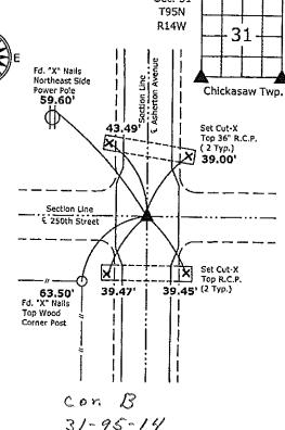
1.) Southwest Corner Section 31-95-14 Set 5/8"Ø rebar w/2"Ø aluminum cap PLS 15525
