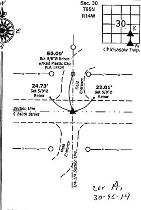
2.) Southeast Corner SW 1/4-SE 1/4 Section 30-95-14 Set 5/8"Ø rebar w/2"Ø aluminum cap PLS 15525
