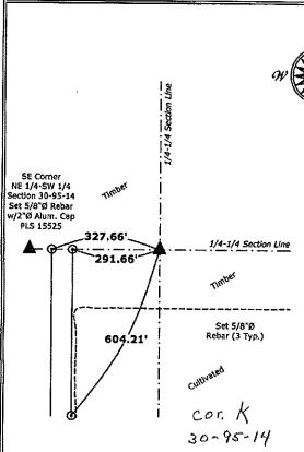
1.) Southeast Corner NW 1/4-SE 1/4 Section 30-95-14 Set 5/8\*Ø rebar w/2\*Ø aluminum cap PLS 15525
