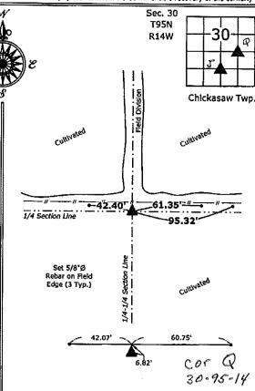
2.) Southeast Corner SW 1/4-NE 1/4 Section 30-95-14 Set 5/8\*Ø rebar w/2\*Ø aluminum cap PLS 15525
