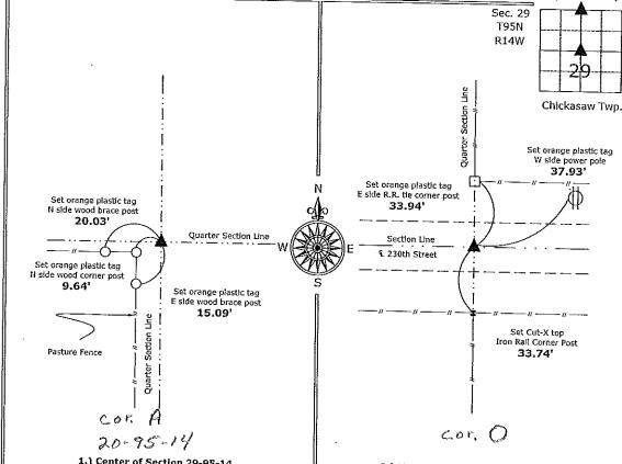
1.) Center of Section 29-95-14 Set 5/8"Ø rebar w/2"Ø aluminum cap PLS 15525
