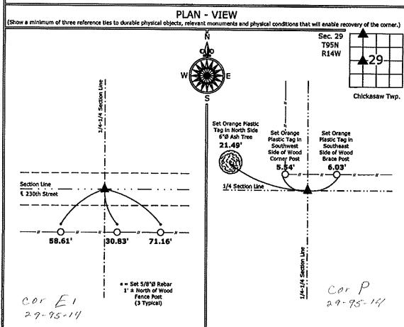
1.) Northwest Corner NE 1/4-NW 1/4 Section 29-95-14 Set 5/8'Ø rebar w/2'Ø aluminum cap PLS 15525 2.) Southwest Corner SE 1/4-NW 1/4 Section 29-95-14 Set 5/8\*Ø rebar w/2\*Ø aluminum cap PLS 15525
