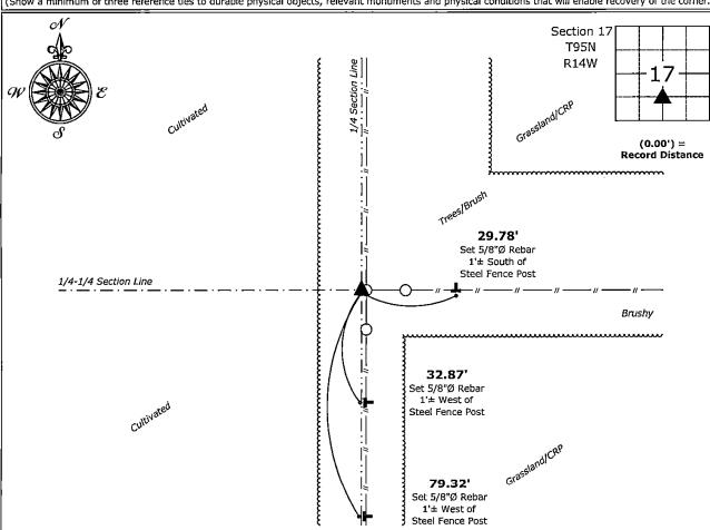
Northwest Corner of the SW 1/4 - SE 1/4 of Section 17-95-14 Set 5/8"Ø Rebar w/2"Ø Aluminum Cap PLS 19211
