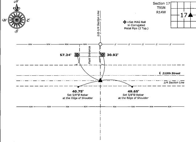
Northeast Corner of the NW 1/4 - SE 1/4 of Section 17-95-14 Set 5/8"Ø Rebar w/2"Ø Aluminum Cap PLS 19211
