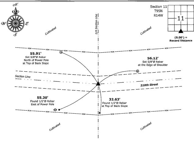
South 1/4 Corner of Section 11-95-14 Set 5/8"Ø Rebar w/2"Ø Aluminum Cap PLS 19211
