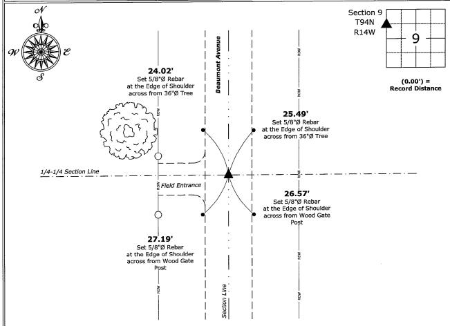
Southwest Corner of the NW 1/4 - NW 1/4 of Section 9-94-14 Set 5/8"Ø Rebar w/2"Ø Aluminum Cap PLS 19211
