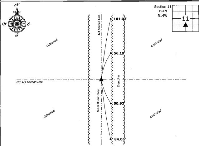
Set 5/8"Ø Rebar at the Edge Tree Line (4 Typical)
